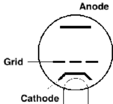
The Cathode emits electrons when heated which will flow to the Anode if a positive voltage (with respect to the cathode) is applied. Current will not flow in the reverse direction.
