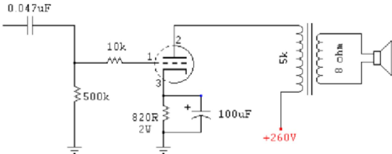
This triode is operating as an amplifier. The Characteristics have been reviewed and components chosen to ensure the device is operating in a linear region. The circuit is implementing Cathode bias to achieve this.
