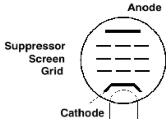
The Cathode emits electrons when heated which will flow to the Anode if a positive voltage (with respect to the cathode) is applied. Current will not flow in the reverse direction.
