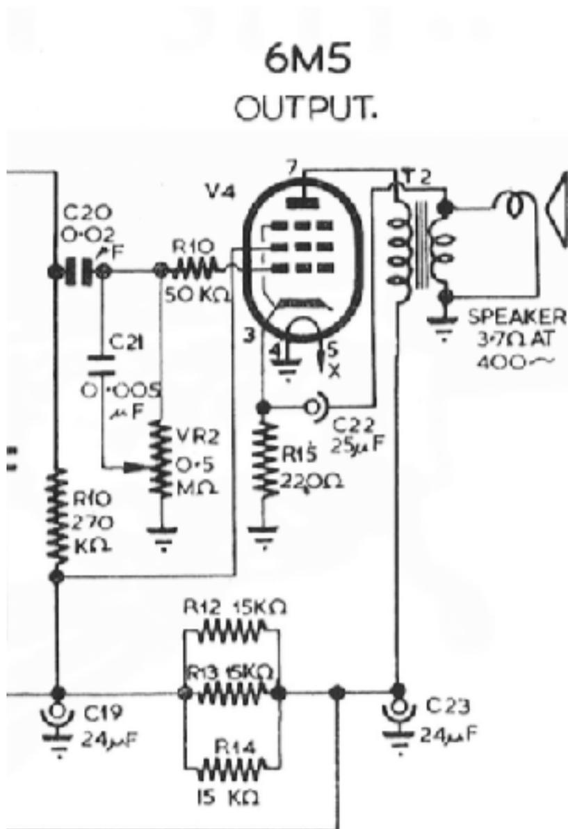
This Pentode is configured to operate as an amplifier. The Characteristics need to be reviewed and components chosen to ensure the device is operating in a linear region.
